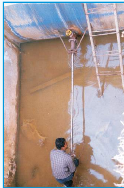
Water Flow Measurement Using Pitot Tube.
